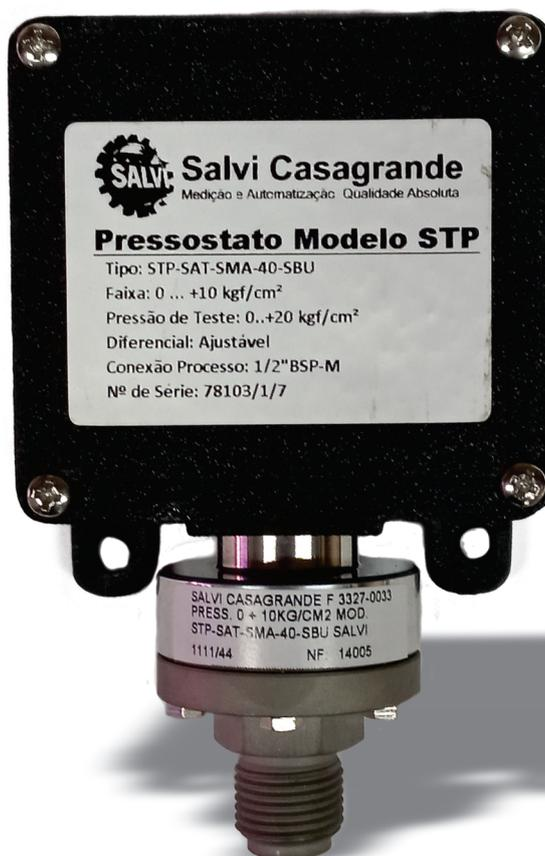
PRESSOSTATO CONSTRUÍDO EM CAIXA À PROVA DE TEMPO, CONTATO ELÉTRICO REVERSÍVEL CAPACIDADE 10 AMPERES 250 VOLTS AC, AJUSTÁVEL, CONECTOR INOX, DIAFRAGMA BUNA, ROSCA 1/2" BSP MACHO, PARA USO GERAL, MODELO STP-SAT-SMA-40-SBU, ESCALADE 0A+10 KGF/CM<sup>2</sup>. - MARCA SALVI.
